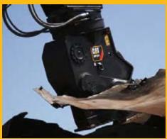
Tank Shear (TS) Jaw
