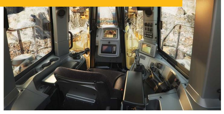
The D9T cab is designed and equipped for operator productivity, safety and comfort. The standard isolation-mounted cab reduces noise and vibration. Overall operator sound levels have been reduced by 2 dB(A). Large windows, tapered hood, and notched fuel tank provide excellent visibility to all sides of the machine and around the job site.
